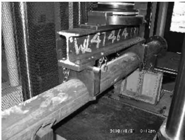
Figure 2 | Pipe section under test showing load application through a spreader beam.
