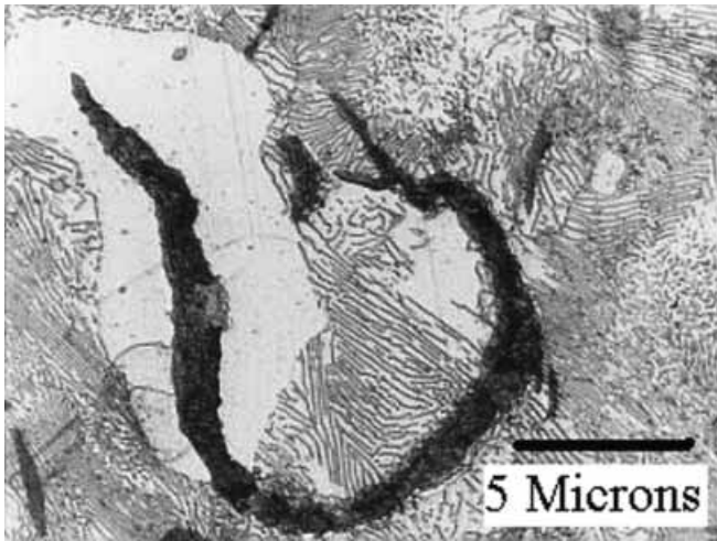
Figure 5 | Photomicrograph depicting regions of pearlite within the etched microstructure.
